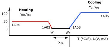
mode is set with 1A03. As the system moves into heating mode, heating airflow increases until it reaches the maximum heating output (1A04), typically 30 to 50% of maximum cooling airflow.
