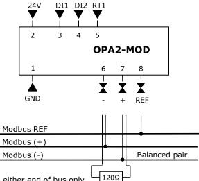
On last node on either end of bus only  $\frac{120\Omega}{}$  connect  $120\Omega$  termination resistor between A and B (D0 and D1)
