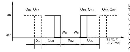
Legend Τ, υ Input signal OSH Offset heating/direct O<sub>SC</sub> Offset cooling/reverse  $X_{DZ}$ Dead zone X<sub>SBY</sub> Economy set point shift Wн Set point heating/reverse Wc Set point cooling/direct Q<sub>C</sub>, Q<sub>D</sub>Binary sequences cooling/direct Q<sub>H</sub>, Q<sub>R</sub>Binary sequences heating/reverse
