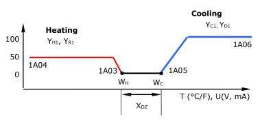
reaches the maximum heating output (1A04), typically 30 to 50% of maximum cooling airflow.
