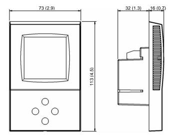
Space required in flush mounting box:  $(H \times W \times D)$ 60 x 50 x 32mm (2.4 x 2.0 x 1.3 in.)
