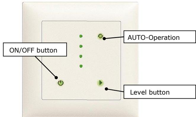
The operating modes are activated after 2 seconds. This prevents unnecessary switching when setting the device. The Level-indication and buttons light up in green or blue depending on the type of device.
