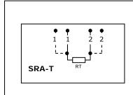
Platinum film and NI1000 sensors use double contacts in order to compensate conductor resistance.
