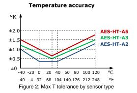
Note on accuracy: Allow 1 hour after power up for compensation swing until described accuracy is reached.
