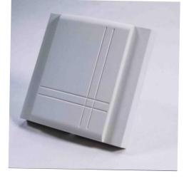
The transmitter measures the temperature by the use of a precision sensing element. The microprocessor samples the temperature once per second. It calculates an averaging signal over a preset number of seconds and generates an output signal based on lower and upper signal range values. Standard range is -40...60°C (-40...140°F) and 10 seconds average. The measuring range and the averaging samples may be customized with the programming tool.
