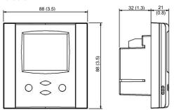
Space required in flush mounting box: (H x W x D)  $60 \times 50 \times 32 \text{ mm}$  (2.4 x 2.0 x 1.3 in.) Distance for mounting screws: Horizontal and vertical: 45 to 63 mm (1.8 to 2.5 in.)
