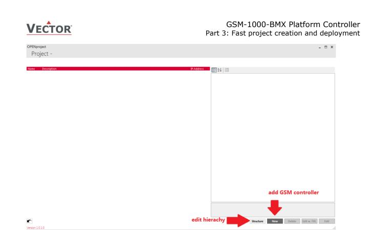
Your GSM controller's IP needs to be filled in correctly. The click "edit" at the bottom right corner to enter the application assignment page.
