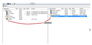
At this point the HMTL page is ready for point bindings and the graphic pages will be seen after uploading the program to your controller.
