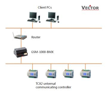
As you can see, it's quite easy to deploy. With RS485 based BAC or MOD protocols a series of TCX2s will be integrated. Have the GSM-1000-BMX placed in your local network then all PC terminals within the range can visit it.
