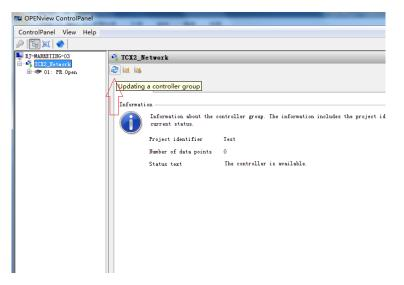
4. After the updating was done, expand the controller icon in the tree left and login using"0007" to your project.
