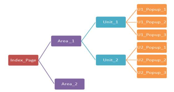
The Vector project template has a four level hierarchy. The "Index\_Page" contains area buttons to enter each area. In each area the chosen applications will be generated dynamically based on your assignment in OPEN Project Builder.
