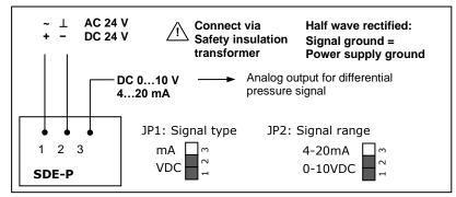
**Signal range selection:** Both JP1 and JP2 must be placed for current or voltage signals. For different ranges than 4-20mA or 0-10VDC, adjust OP01 and OP02.
