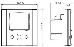
Space required in flush mounting box:  $(H \times W \times D)$  60 x 50 x 32 mm (2.4 x 2.0 x 1.3 in.) Distance for mounting screws: Horizontal and vertical: 45 to 63 mm (1.8 to 2.5 in.)
