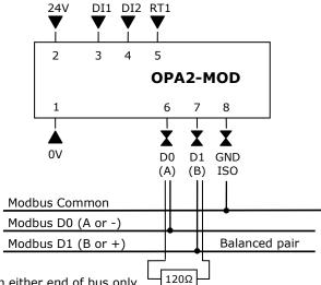
On last node on either end of bus only connect 120Ω termination resistor between A and B (D0 and D1)
