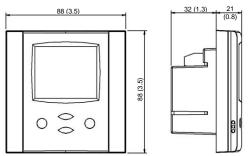
Space required in flush mounting box: (H x W x D) 60 x 50 x 32mm (2.4 x 2.0 x 1.3 in.) Distance for mounting screws: Horizontal and vertical: 45 to 63mm (1.8 to 2.5 in.)
