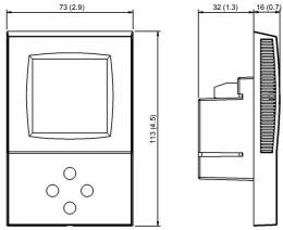
Space required in flush mounting box:(H x W x D) 60 x 50 x 32mm (2.4 x 2.0 x 1.3 in.) Distance for mounting screws: Horizontal and vertical: 45 to 63mm (1.8 to 2.5 in.)
