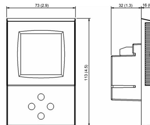
Space required in flush mounting box: (H x W x D) 60 x 50 x 32mm (2.4 x 2.0 x 1.3 in.)
