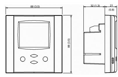
Space required in flush mounting box: (H x W x D)  $60 \times 50 \times 32$ mm (2.4 x 2.0 x 1.26 in.)
