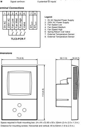
Fan Coil Controller TLC3-FCR-T-U-230-W51
