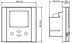
Space required in flush mounting box: (H x W x D) 60 x 50 x 32mm (2.4 x 2.0 x 1.26 in.) Distance for mounting screws: Horizontal and vertical: 45 to 63mm (1.8 to 2.5 in.)
