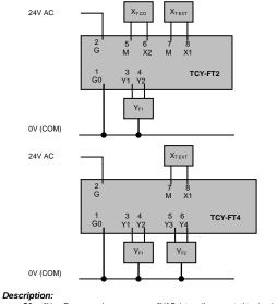
GO 0V Power supply: 0VAC, internally connected to signal common G 24V Power supply: 24VAC м 0V Signal common: Common 0 potential for analog inputs and analog outputs. X1 RT External temperature input: NTC 10kΩ @ 25°C (77°F)
